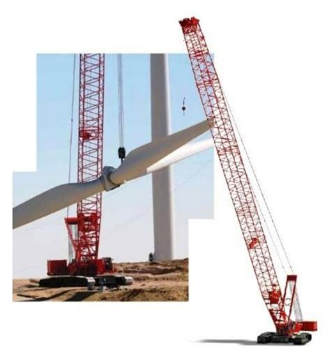
Max. Lifting capacity - 400 Tons Heavy Lift Boom - 96.0m Fixed Jib on Heavy Lift Boom - 105.6m Luffing Jib On Heavy Lift Boom – 138.0m Engine Output - Cummins 372 kW @ 1800 rpm Swing Speed – 0-2.2 rpm
